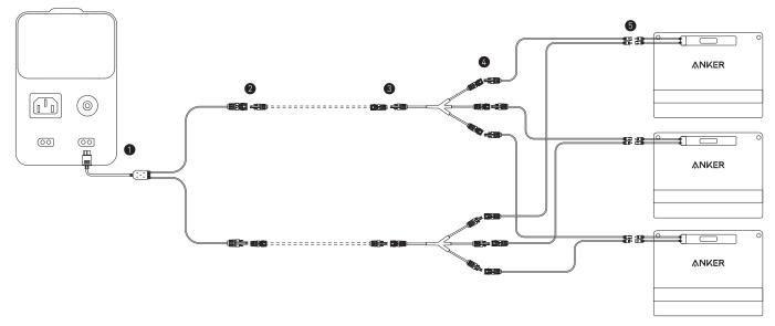
\*If the solar panel is far from the power station, you can purchase the Anker SOLIX Solar Panel MC4 Charging Cable as an
